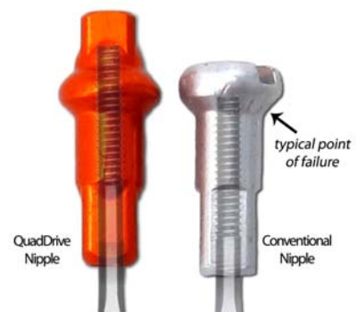
Size your spokes 2.3mm longer than for a conventional nipple. This allows the threads to pass deep into the head of the nipple, the typical weak point in a conventional alloy nipple.
